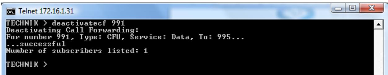
A screenshot of a Telnet window titled 'Telnet 172.16.131'. The prompt is 'TECHNIK >'. The user has entered 'deactivatecf 991'. The output shows 'Deactivating Call Forwarding:' followed by 'For number 991, Type: CFU, Service: Data, To: 995...' and '...successful'. Finally, 'Number of subscribers listed: 1'. The prompt is now 'TECHNIK >'.
