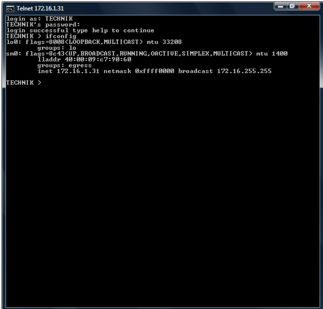
A screenshot of a Telnet terminal window titled 'Telnet 172.16.131'. The terminal shows a login sequence for user 'TECHNIK'. After the user enters their password, they type the command 'ifconfig'. The terminal displays the following output:
