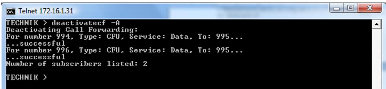
A screenshot of a Telnet window titled 'Telnet 172.16.131'. The prompt is 'TECHNIK >'. The user has entered 'deactivatecf -A'. The output shows 'Deactivating Call Forwarding:' followed by two lines: 'For number 994, Type: CFU, Service: Data, To: 995...' and '...successful'. Then another line: 'For number 996, Type: CFU, Service: Data, To: 995...' and '...successful'. Finally, 'Number of subscribers listed: 2'. The prompt is now 'TECHNIK >'.
